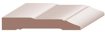
**E117** 9/16 x 3-1/2 **Colonial Casing/Base** (use with E190 to create a wider casing)
